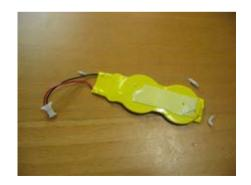
Cut open the plastic jacket to expose the two cells.
