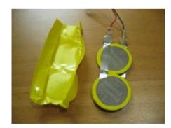
Separate the two metal strips from the old cells. This will take some effort so as they are welded on strong. Just be careful not to actually break the strips. Notice how mangled they can get after separation!
